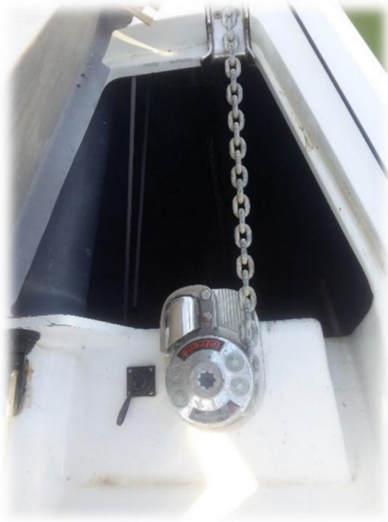
5 Bow Area: staple, anchor & 50m chain, picture from the locker
