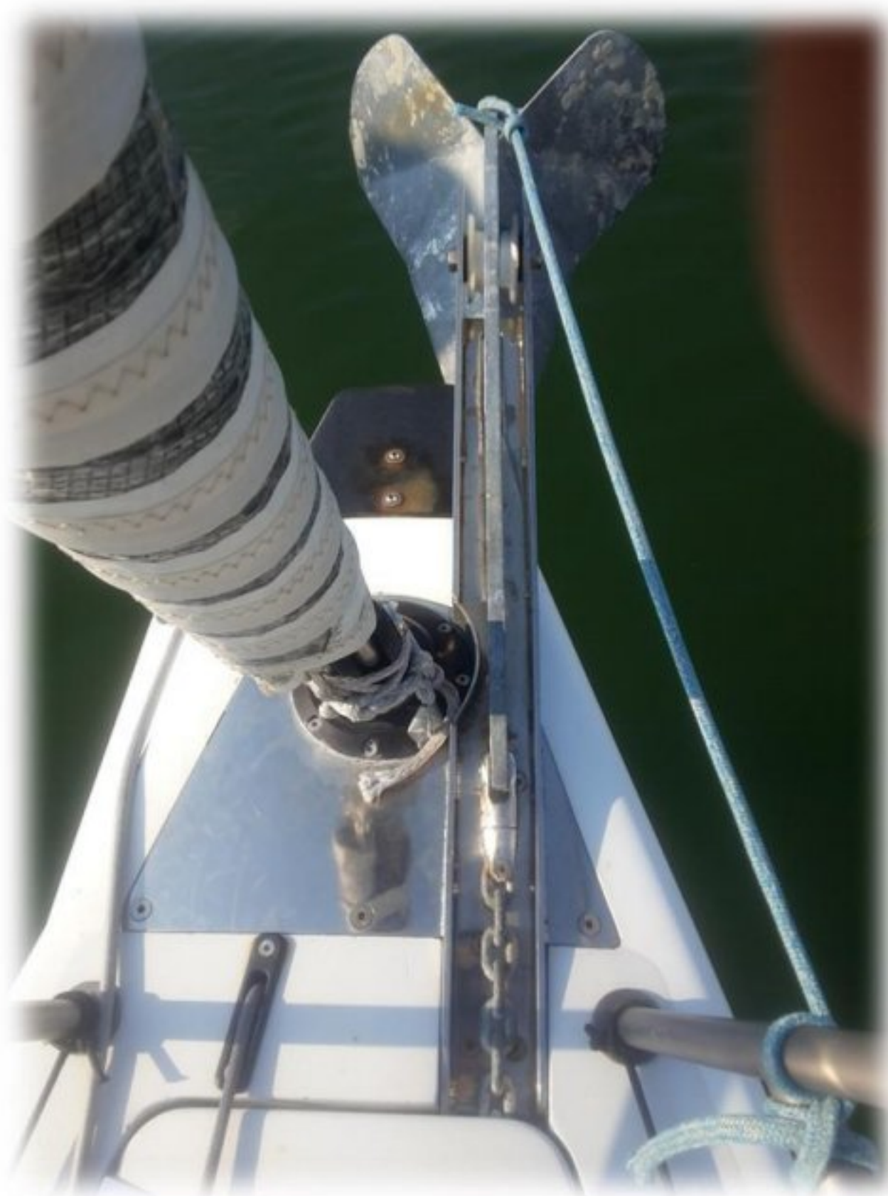
5 Bow Area: staple, anchor & 50m chain, picture from the locker
